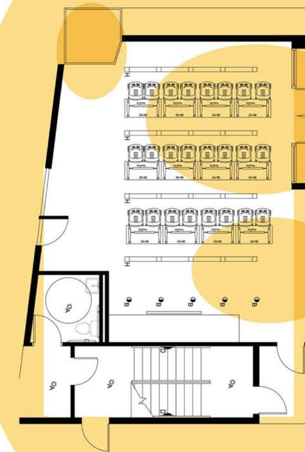
Daytime: Photosensors Turn Lights Off
